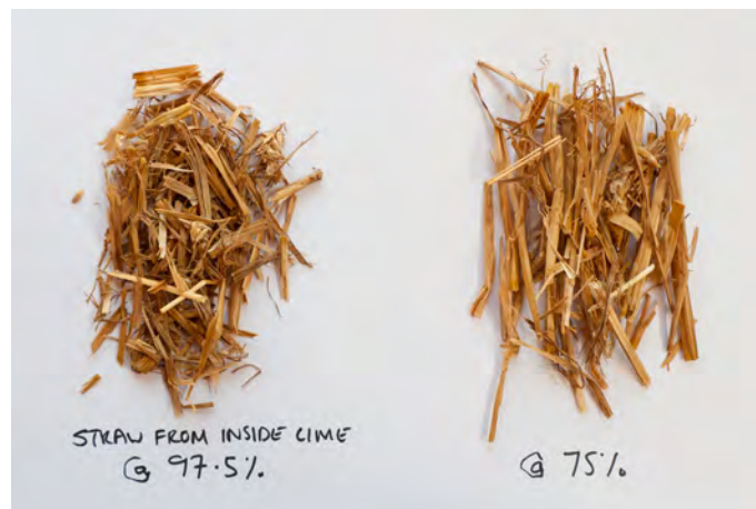
Fig.51 Straw from inside the lime plastered lumps
