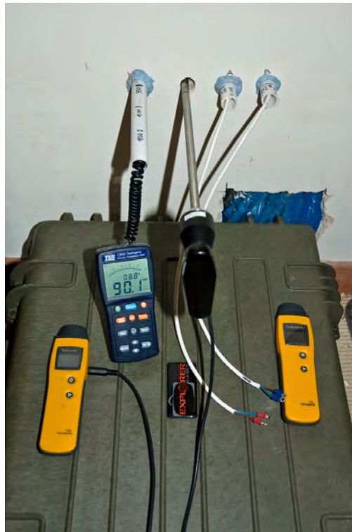
Fig.31 Setup for initial tests of the new probes The devices inserted in the wall are as follows (L to R): TES 1365 RH and Temperature meter, 'Bailemaster' probe and the two wood block probes. In the foreground is the 'Bailemaster' meter, and the Timbermaster meter for reading the moisture content of the timber bullets on the probes.
