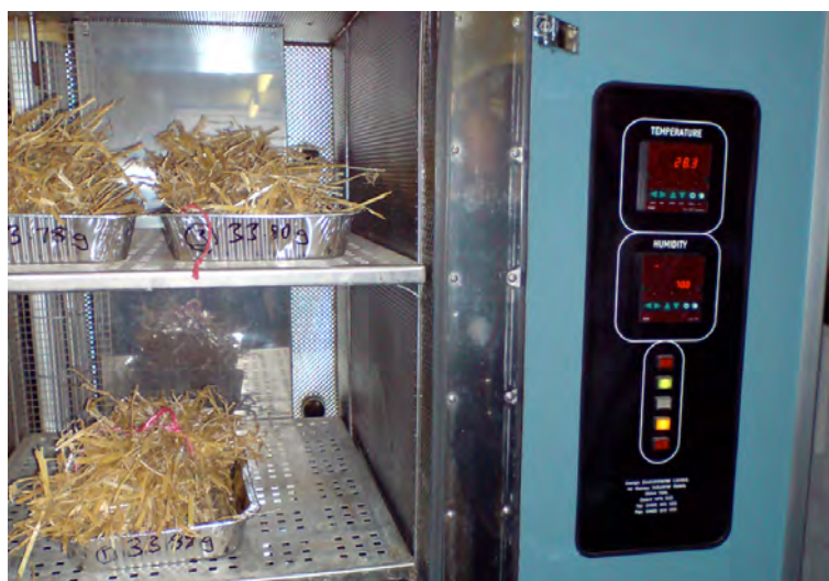
Fig.38 Samples of straw in the Environmental Chamber
