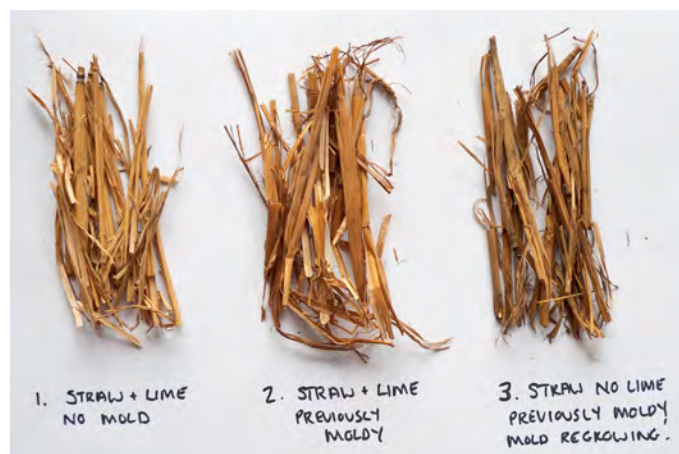
Fig.50 Three samples from desiccators at 97.3% RH
