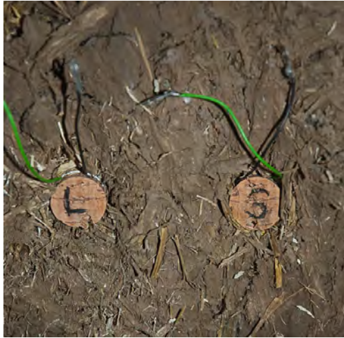
Fig.A24 Probes installed in earthen render
