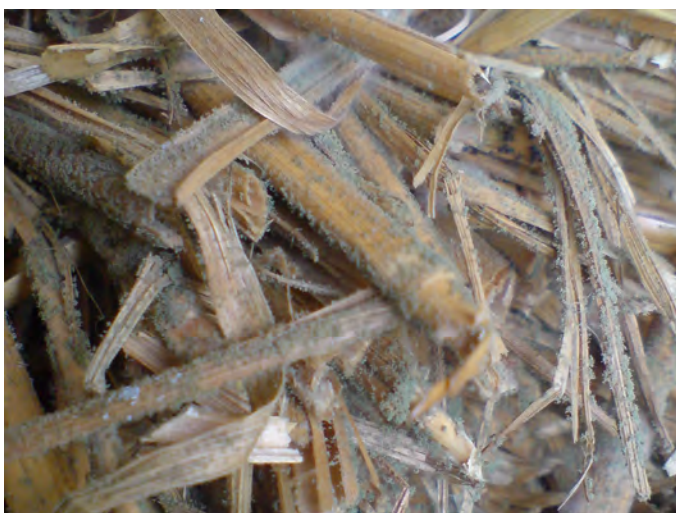
Fig.45 Mould growing of straw after three months at 97.6% RH
