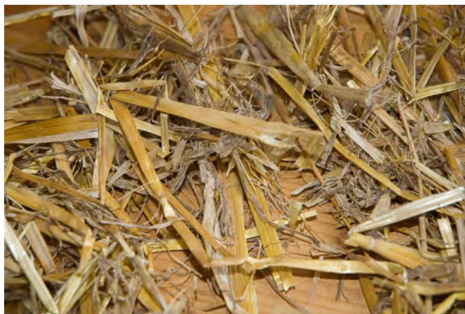
Fig.94 Straw from the damp wall at the Totnes House, after drying
