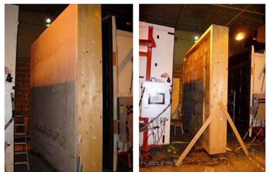
Figure 5 Prefabricated ModCell panel and Guarded Hot Box facility at the BBA, Garston, UK.
