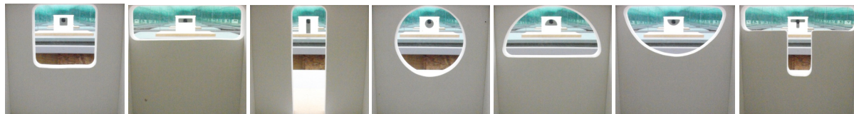
Fig.1: Square, wide, tall, round, arch, inverted arch, and 'T' window shapes are tested, with equal glazing area.
