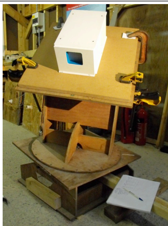
Fig.8: Using a slide projector as a fixed 'sun', the heliodon emulates the tilt and rotation of the earth for any given latitude, solar time, and orientation, for the solstices and equinoxes.
