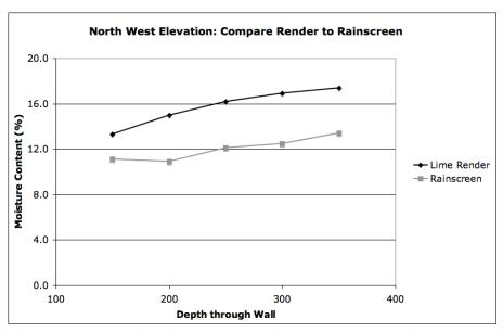
Fig 3. Readings of moisture content from the same position on the ground floor (lime render) and first floor (timber rainscreen) on the Southeast and Northwest elevations of the Totnes house taken on the 8<sup>th</sup> of November 2008
