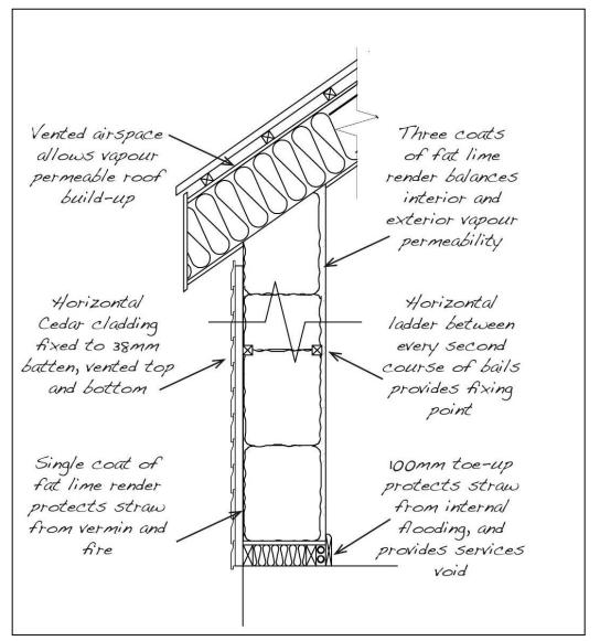
Fig 5. Simplified section through a straw bale wall with a vented timber rainscreen cladding pane
