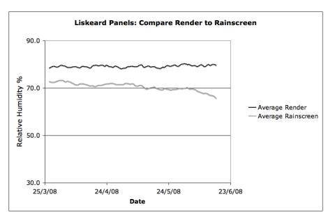
Fig 4.Average readings of relative humidity for two of the panels shown in Figure 2 during April, May and June 2008. The higher trace being from the rendered panel, the lower is from the panel protected by a rainscreen.
