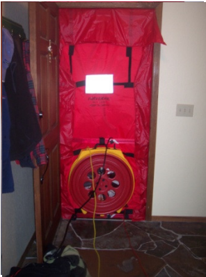
Figure 1: Blower Door setup.
