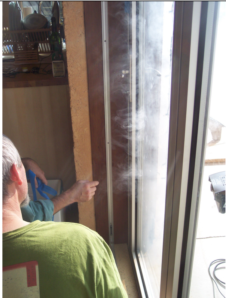
Figure 30: Visual illustration of fog entering through small leakage area of sliding glass door during house depressurization.
