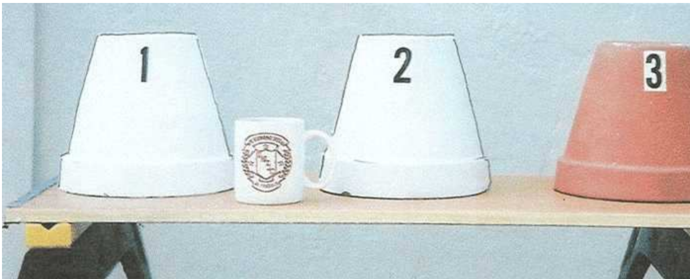
Figure 6. Large clay pots turned upside down exposed to ambient condition in full sun; #1 enamel white; #2 white limewash; #3, natural clay color. Inside temperatures recorded after three hours exposure and subsequent gain in temperature is recorded. Ambient temperature of 94°F.
